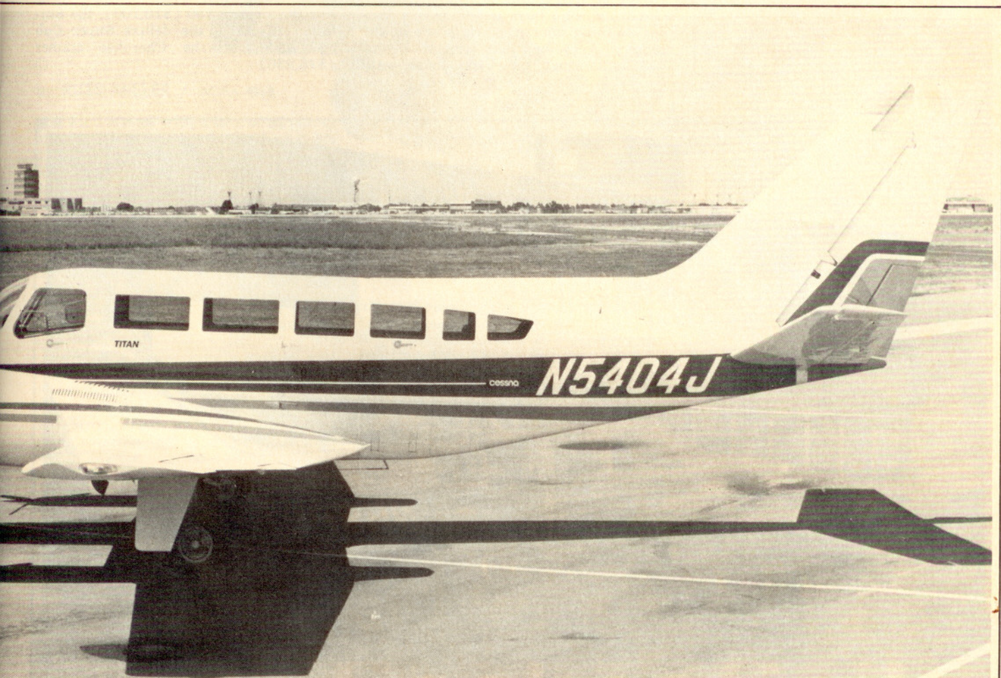
Cessna's turbocharged Titan looks much like the 441 and shares certain of its features: trailing-link landing gear; Fowler-type flaps; and a wet-wing design, using metal-to-metal bonding.
