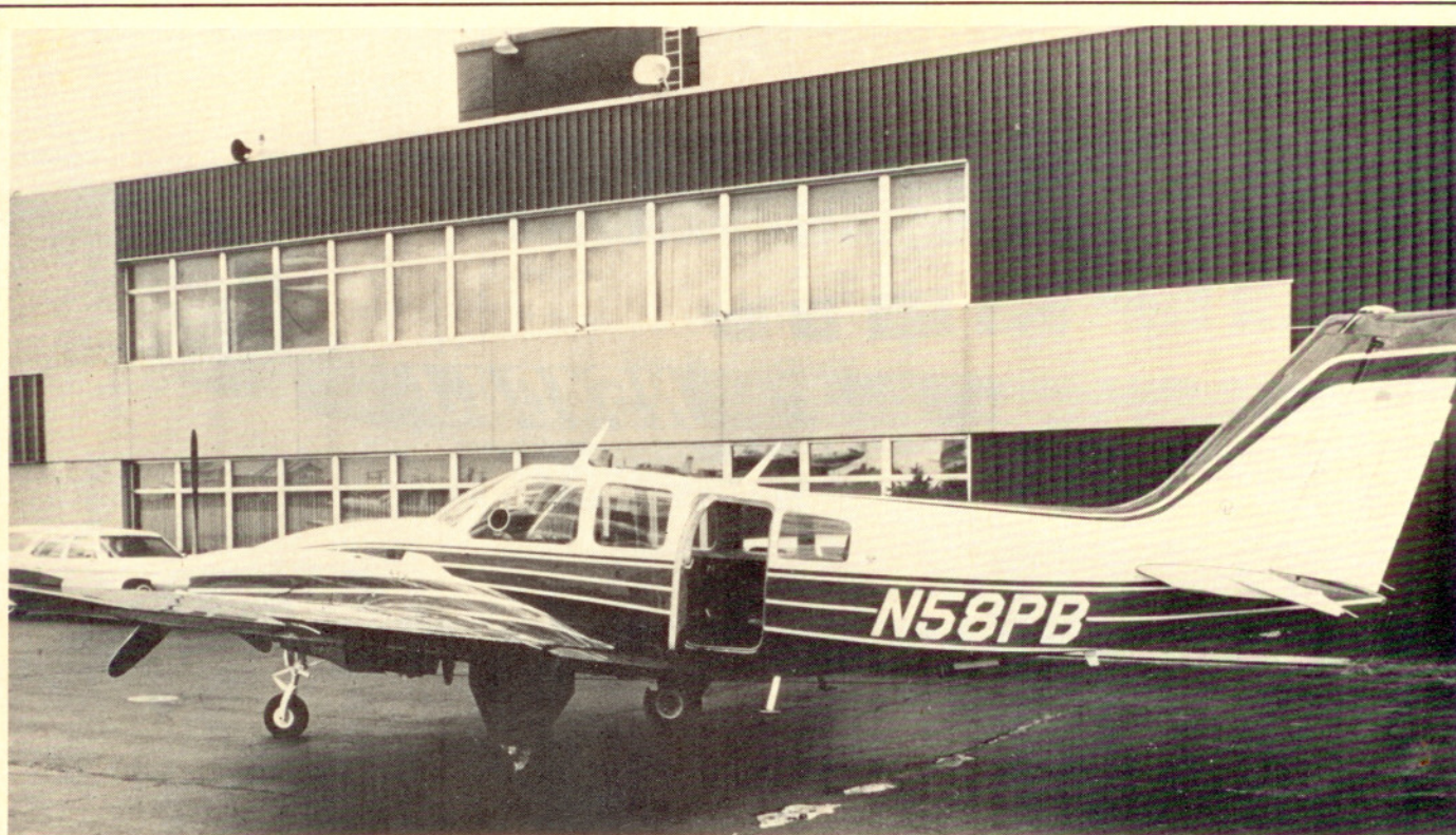
At 65% power at 20,000 feet, Beech's pressurized Baron cruises at 232 mph for more than 1,000 miles. At a flight altitude of 21,000 feet, cabin altitude holds at a comfortable 9,800 feet. Photo by the author.
